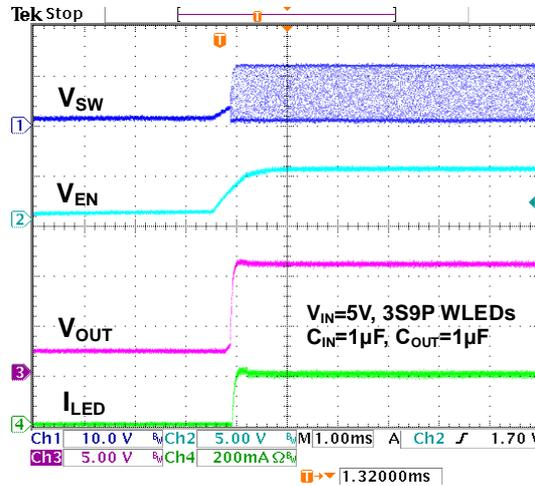
Figure 5. Enable Startup Response Waveforms
