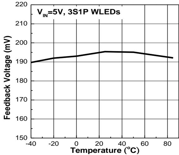
Figure13. Feedback Voltage vs. Temperature.
