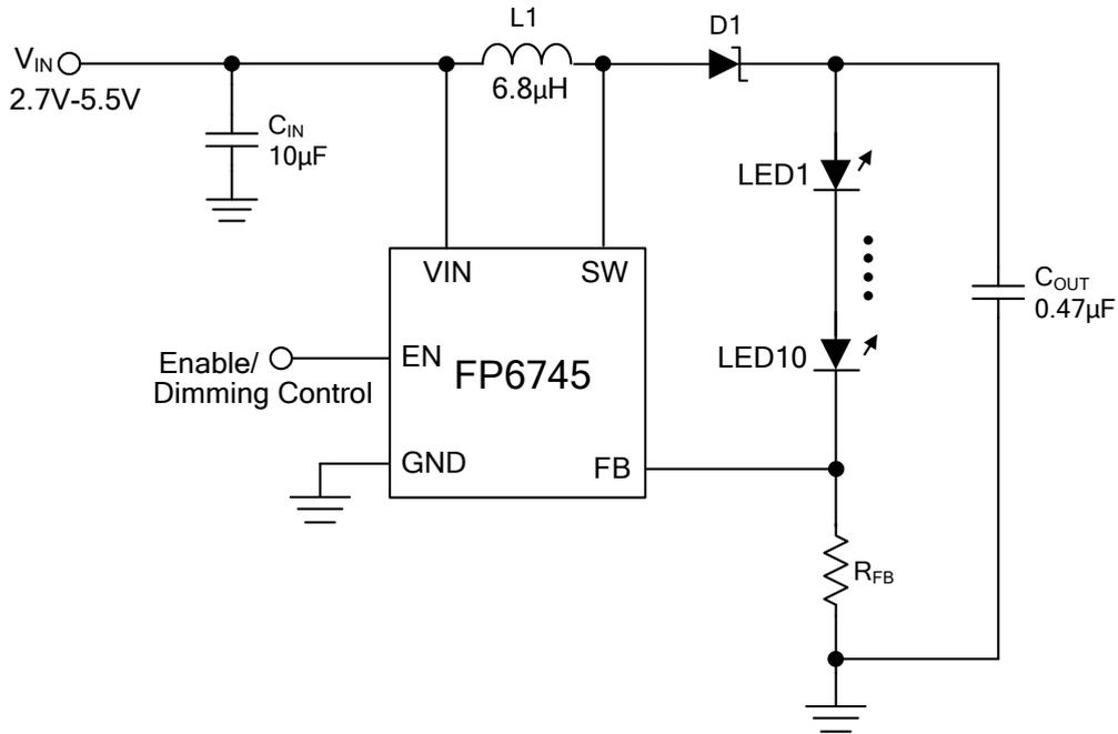
Figure 2. Typical Application Circuit of FP6745
